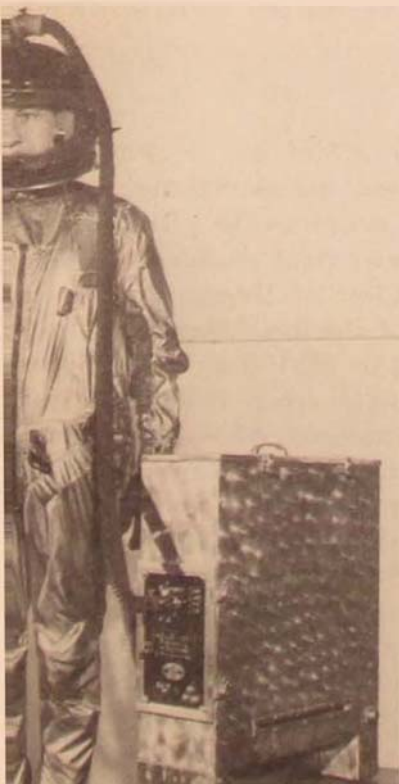
A modified MC-2 suit is shown in combination with a recirculating oxygen-conditioning system. This unit has a cooling capacity of 10,000 British thermal units (BTU) for heat removal during the re-entry period of flight. The exhaled water and perspiration are also utilized for cooling purposes.
